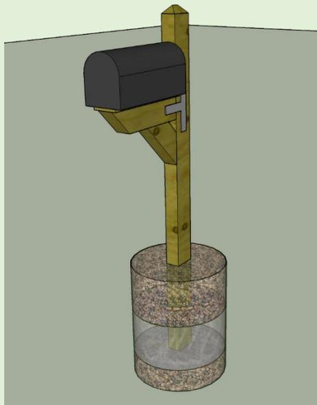
The finished mailbox will sit 42in above the ground and 7in back from the curb. It is anchored 24in below ground. This is within guidelines recommended by USPS
